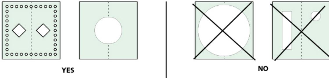
Finally, in determining the cut size of the lamp material, account for the 1/8" laminate border that is required around the entire perimeter of the lamp. This is a critical accommodation for instances where the lamp must fit within a confined frame or area.
