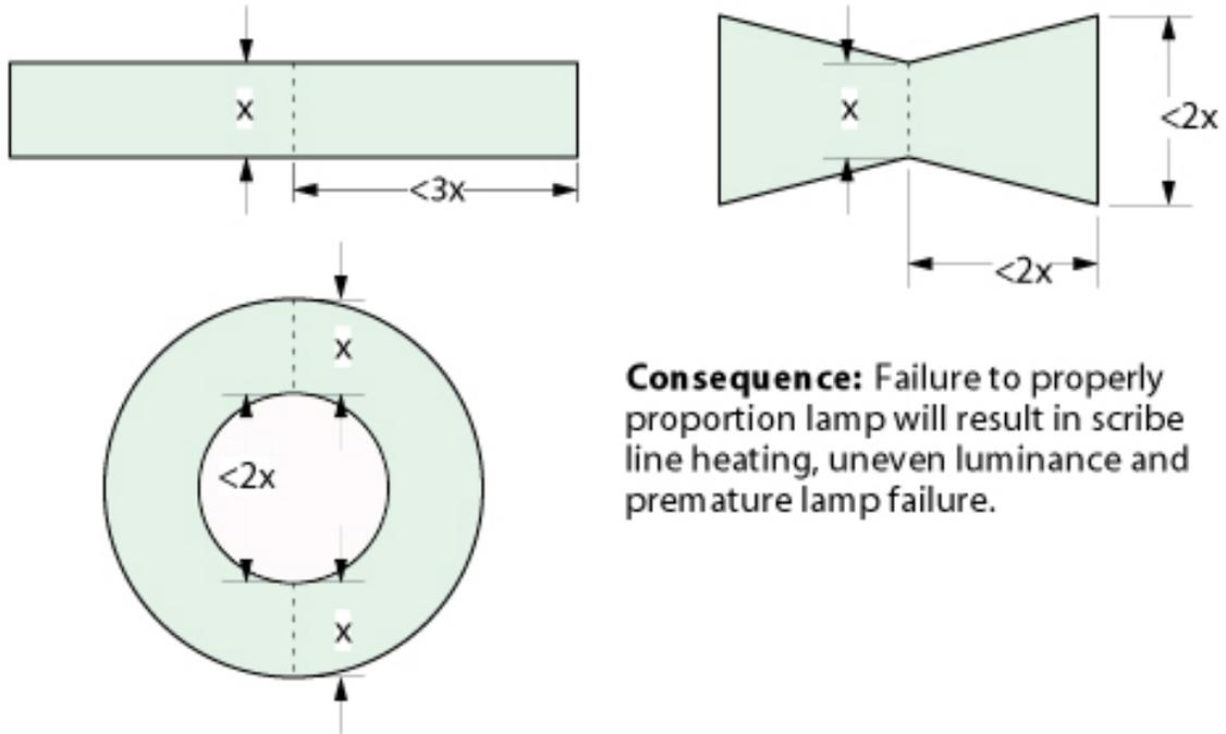
**Consequence:** Failure to properly proportion lamp will result in scribe line heating, uneven luminance and premature lamp failure.
